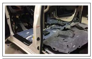
e) Fold the carpet back into the second-row seating area, with the fold in the area of the B-Pillar.
