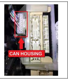
DO NOT unplug the individual CAN connectors. Only separate the entire housing from the JB.
