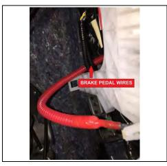
Route the harness around the back side of the connector block, making sure to have the wire behind (bulkhead side) the brake pedal wire harness.
