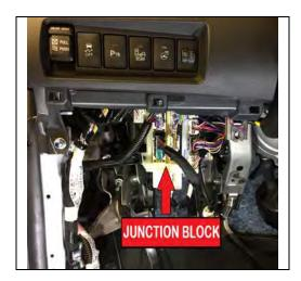
d) Pull the CAN Communication connector housing toward you and separate it from the JB. DO NOT pull by the wires.
