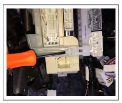
e) Attached on the right side of the JB is a bracket that holds additional connectors. Use a small screwdriver to release the locking tab in the front lower right corner of the JB.
