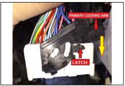
d) Fold the Connector Locking Arm to the locked position by first releasing the latch on both sides and then pivoting the arm to the locked position.
