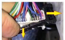
e) Slide the Connector Locking Arm off the connector by first pulling outward at the rear of the arm on both sides, about 1/4" (6mm). This should be just enough for the slots on the Primary Locking Arm to clear the pins on the connector.
