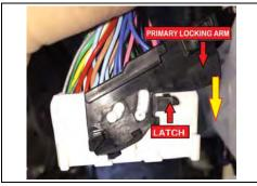
d) Fold the Connector Locking Arm to the locked position by first releasing the latch on both sides and then pivoting the arm to the locked position.
