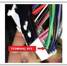
c) Turn the connector around to view the wire side of the connector. Locate the wire that is plugged into terminal #13. It will be a light green color.
