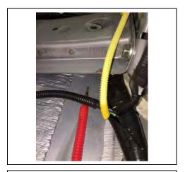
c) Route the terminal end of sub-harness #7 (shown in red) under the sheet metal brace at the B-pillar on the RH side. Start at the rear of the brace and push the wire through the space between the brace and floorboard until it is reachable from the front side of the brace.
